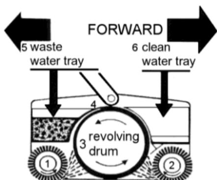
Two counter-rotating brushes (1 and 2) throw the soiled water on to the revolving drum (3), from there it is fed into the waste water tray (5) by means of a stripper blade (4).
