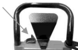
Make sure that the on/off switch is in the "ON" position - only for models A, S, S-M and B.
