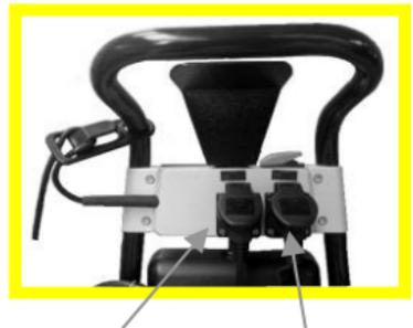
Pump socket    Motor socket
