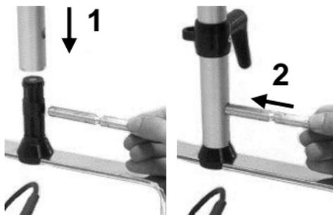
Place the handle (1) on the plastic handle connector on the fork and push connecting pin (2) through to locate handle.
