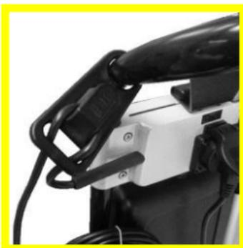
Place for an extra protection the main cable in the cable safety.
