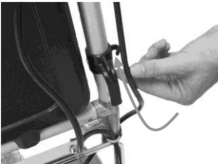
Push the mains cable into the purpose-made hooks on the handle. This will avoid the cable being run over by the revolving brushes
