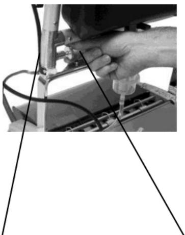
Place the loop handle on the aluminium handle connectors and fit spring loaded bolts to locate.
